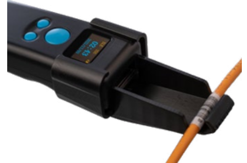
Bluetooth®-enabled handheld barcode scanner and pre-labeled cable
